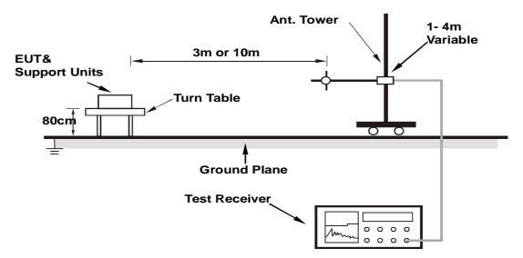
Note: Cable on the RGP must to be insulated.
