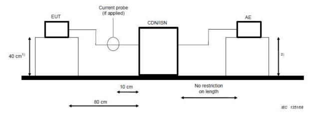
AE = Associated equipment EUT = Equipment under test
