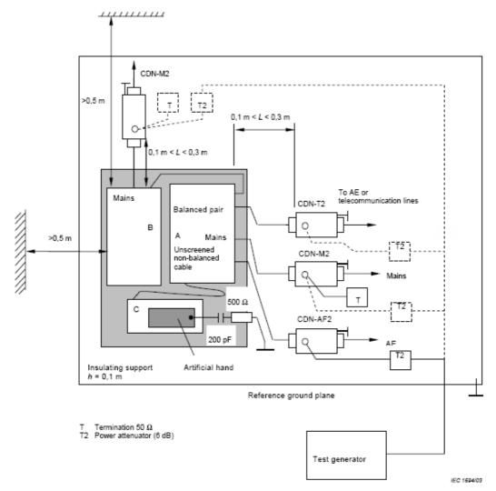
**Note:** 1.The EUT clearance from any metallic obstacles shall be at least 0,5 m.
